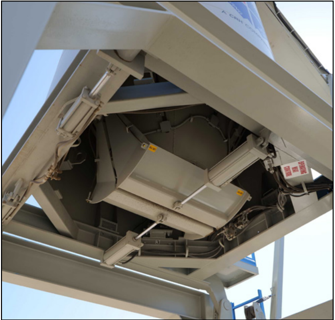
There are two independently driven, remotely controlled clam style main gates.
