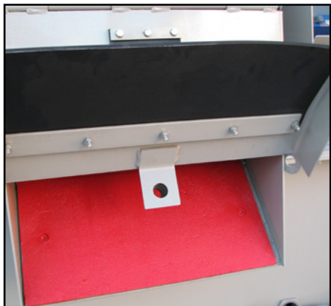
Gencor's heavy-duty replaceable wear liners in all the right places provide longer wear and lower maintenance.
