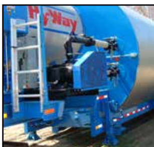
Mounted Unloading Pump
