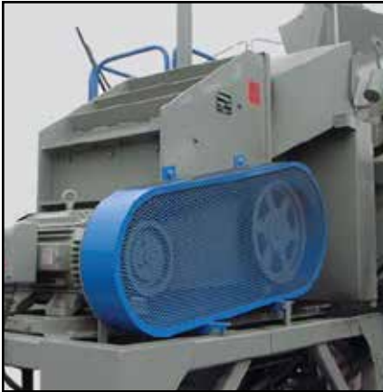
The Hammermill Crusher is hinged for easy access to mill interior by means of a hydraulic power unit.
