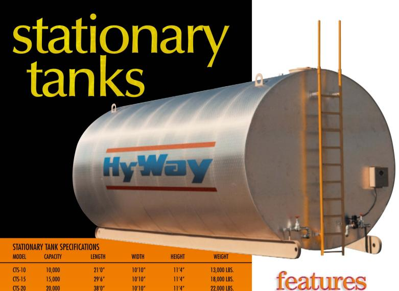
Stationary tanks feature a high-efficiency, close-wound, serpentine coil for increased oil circulation and better heat transfer. 1/4" buttwelded steel plate forms the rugged shell construction of the tank with 4' of fiberglass insulation on the shell to reduce conductive heat loss. A series of integral saddles mounted on heavy twin 25 pound beams form the support frame which is easily set to grade or adaptable to concrete foundations. To ensure all-weather protection and durability,
