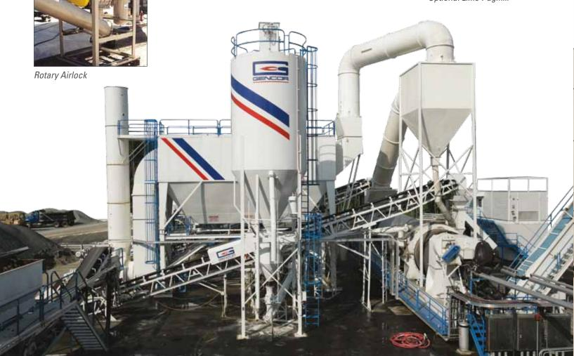
Each additive system is sized per application to assure optimum mix design quality and to meet the tightest state and DOT specifications. Mineral silos are available from 200 to 900 bbl capacity for addition of fly ash, dust, lime, or other mineral additives to the asphalt product.
