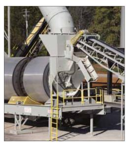
The oversized feed breechings allow for smooth uninterrupted flow of material while also providing a large knock-out area to minimize dust carry-out. The breeching is equipped with replaceable Ni-hard wear liners, vibrator and pneumatically operated calibration divert chute.
