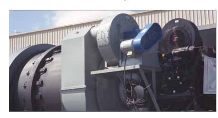
Gencor's patented combustion T-flights reduce energy costs by allowing conductive and convective heat transfer to the aggregates while creating an isolated combustion zone free from flame impingement.
