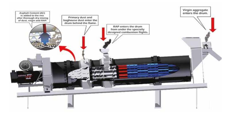
This special flighting allows the RAP material to cascade around the combustion zone absorbing conductive and convective energy. The heat from this action releases internal moisture before it enters the mixer. RAP, virgin aggregate and baghouse dust combine in the mixing zone, away from the direct radiant zone. Asphalt cement (AC) is then added into a thoroughly dried mixture of primary dust, virgin aggregate and RAP to form a fully coated and homogenous mix before exiting the drum.
