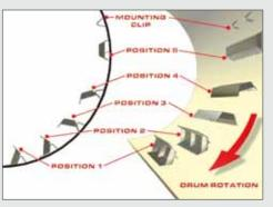
Gencor's patented Converta-flight™ is a 5-way adjustable veiling flight that provides easy adjustment of material veil in the drying section for highly efficient energy utilization and precise control over exhaust gas temperatures especially with RAP, RAS and Warm Mixes. Flight position 5 protects the drum shell against friction and blind wear spots totally eliminating the need to remove the flights from the drum.
