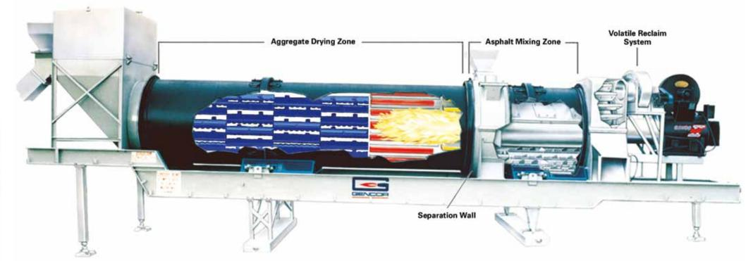
The isolated mixing section is located behind the burner so there is no chance of liquid asphalt coming in contact with the burner flame. This means there is no oxidation of the asphalt, no degradation of the mix, and no asphalt vapors entering the exhaust gas stream. Vapors generated in the mixing section are pulled through the burner by a patented volatile reclaim system and consumed as fuel. There are no odors or blue smoke emissions to pollute the environment.
