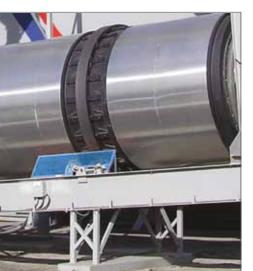
Gencor's **Skid Package** provides solid drum support eliminating the need for concrete foundations.
