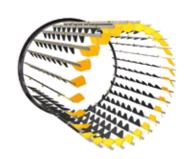
The Gencor discharge wheel is made of abrasion resistant steel paddles that are adjustable and replaceable. The wheel design reduces energy demand on the drum drive system and eliminates segregation of the mix.
