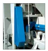
Gencor feeders are driven by an eddy current motor drive system which assures precise speed control at varying production rates using a standard motor coupled with a variable speed torque converter. (optional Variable Frequency Drives are available) Standard features include tail shaft tachometer.
