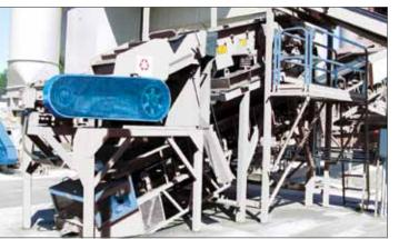
The crusher top is hinged for easy access to mill interior utilizing the manual hydraulic power unit to actuate the opening of crusher for servicing.
