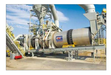
Gencor has demonstrated the effectiveness of the new A.R.E. option with some of the largest asphalt producers in the United States. These plants run applications in excess of 600 tons per hour with as much as 50% recycle (300 tons per hour) of recycled asphalt.
