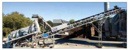
Gencor's **heavy-duty lattice frame** conveyors provide superior support to typical channel frame conveyors. The added strength provides superior support against vibration and wind.
