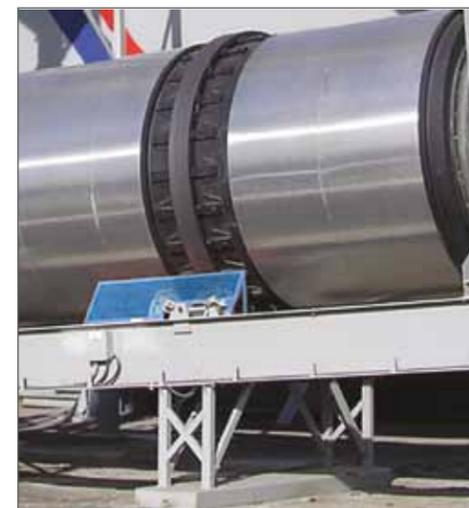
Gencor's **Skid Package** provides solid drum support eliminating the need for concrete foundations.
