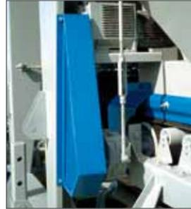
*Gencor feeders are driven by an eddy current motor drive system which assures precise speed control at varying production rates using a standard motor coupled with a variable speed torque converter. (optional Variable Frequency Drives are available) Standard features include tail shaft tachometer.*
