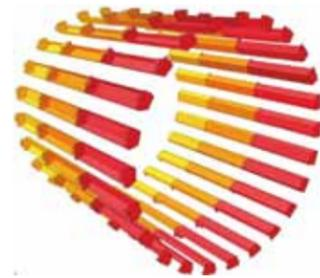
Gencor's **isolated mixing zone** provides for both dry and wet mixing of the materials. The patented flights pull through the mix for thorough homogeneous coating of the aggregates. The kneading action reduces energy demand on the drum drive system and once coated with material virtually eliminates wear associated with typical mixing paddles.
