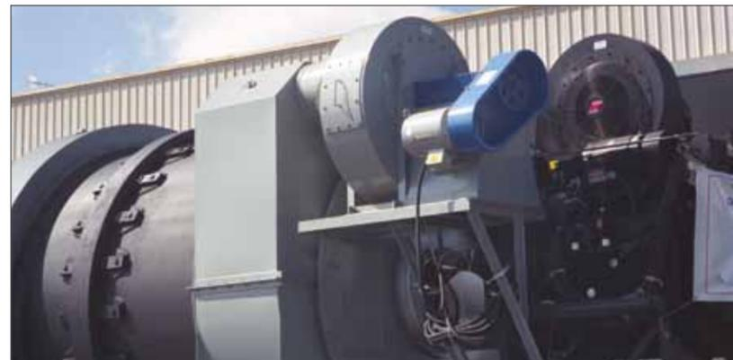
All Gencor **Ultradrums** have oversized drum diameters, in fact the largest in the industry, which provides lower exhaust gas velocities reducing dust carryout and wear on the drum, ductwork and the entire plant exhaust system.
