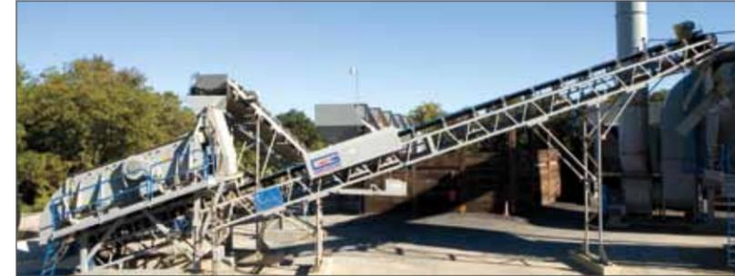
*Gencor's heavy-duty lattice frame conveyors provide superior support to typical channel frame conveyors. The added strength provides superior support against vibration and wind.*
