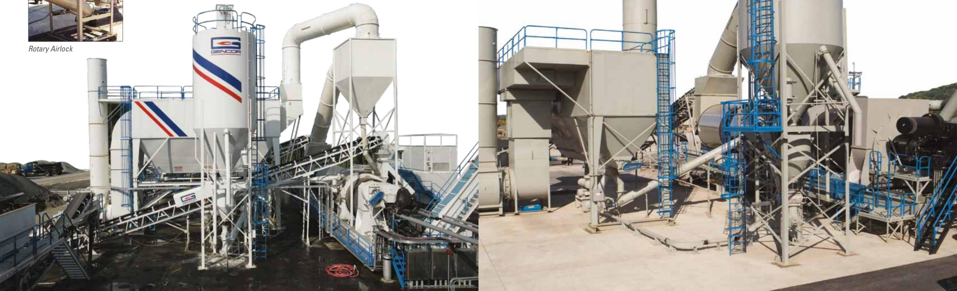
The Ultraflo™ Baghouse Filtration System is the ultimate alternative to pulse jet baghouses. Developed primarily to increase efficiency, reduce maintenance and reduce size and weight, the Ultraflo Baghouse cleaning system from Gencor provides many advantages to typical pulse-jet baghouses.
