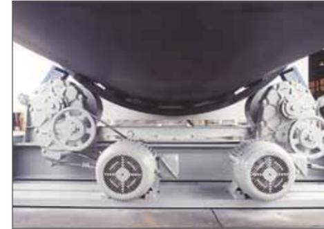
The Gencor **Ultradrum** is driven by a heavy duty friction drive system that evenly distributes positive energy to each tire. Gencor provides four (4) independent drive units to ensure positive traction under any type of climate condition. Friction drive has been proven as more efficient with lower maintenance and lower noise than chain drive systems.
